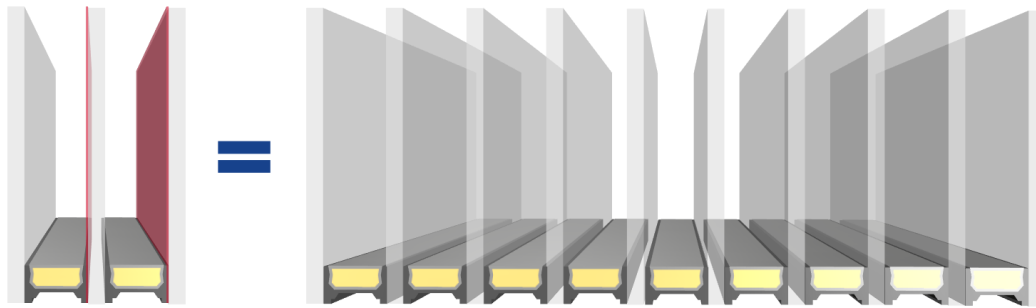
Figure 9 - Equivalent TGU Coated to IGU with No Coatings
